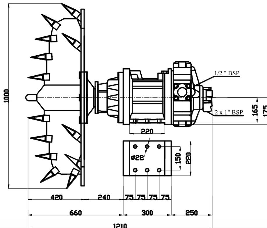
COMPACT SOIL 40 – CLAY 60 – MIXING 80 RPM.
